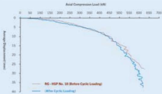
Figure 1: Axial compression load vs. Average displacement of helical pile
