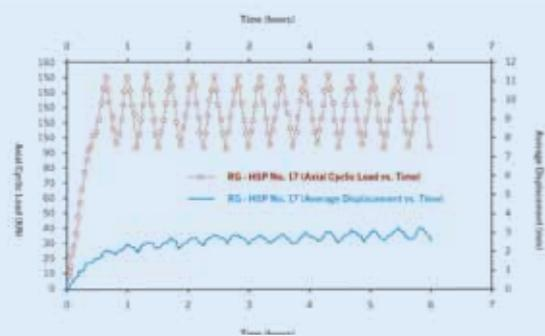
Figure 2: Cyclic loading response of helical pile
