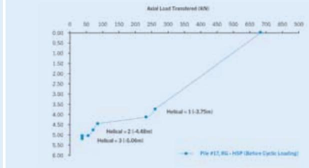
Figure 3: Load transfer to helical plates and grout column
